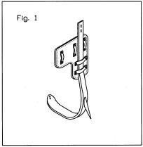
Attach sleeve to leg iron with sleeve loop facing outside of pad (away from the wearer's leg) using the fasteners enclosed. See Fig. 2 ('right' climber shown). Note: Two fasteners (screws, star washers & barrel nuts) must be used to secure each sleeve to each leg iron. Do not over tighten, torque to 25 inch pounds maximum.
